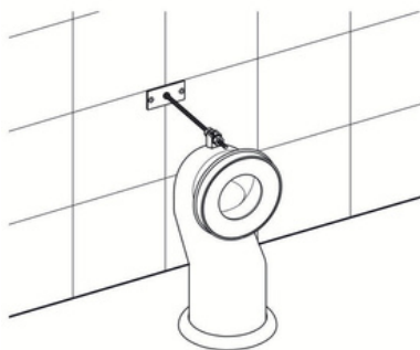
Pipe fitting placement for floor outlet installation.
