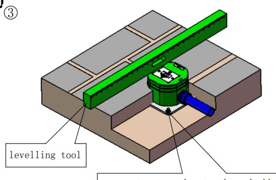
connect water pipe to the embedded part, tight up embedded part to hole bottom with screws, and make sure the cover of embedded part must be same level or 1-3mm lower than floor tile.
