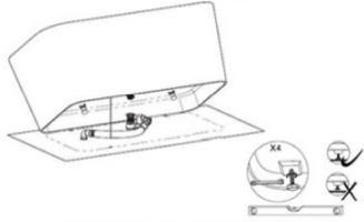
Flexible bathtub feet can be adjusted to make the bathtub standing better on the floor if the floor is unlevel.
