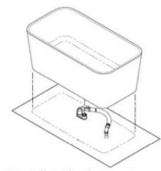
Installate the drain system on the floor.
