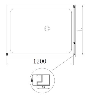
R-BE-2120-120-FFF: L=1165~1180 mm R-BE-2120-130-FFF: L=1265~1280 mm R-BE-2120-140-FFF: L=1365~1380 mm R-BE-2120-150-FFF: L=1465~1480 mm R-BE-2120-160-FFF: L=1565~1580 mm
