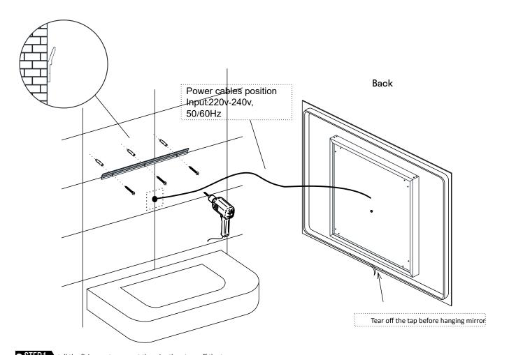
STEP1 stall the fixing parts, connect the wire, then tear off the tap
