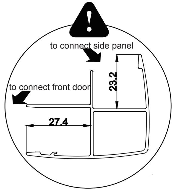
Insert the corner profile into the front fixed glass, and then insert the corner profile into the side panel
