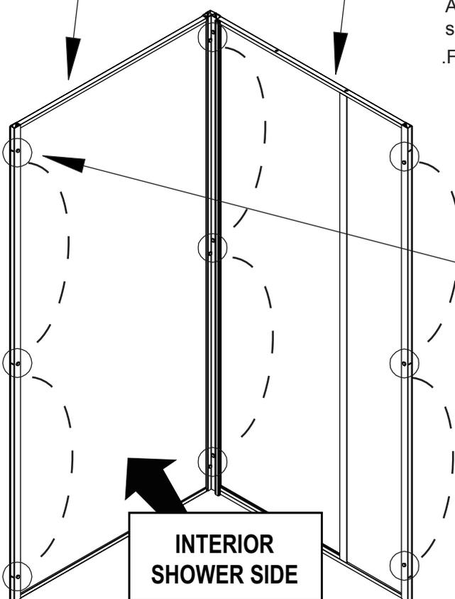
Adjust the level. Drill holes at the wall profile and corner profile separately with  $\Phi 3.2$  screws
