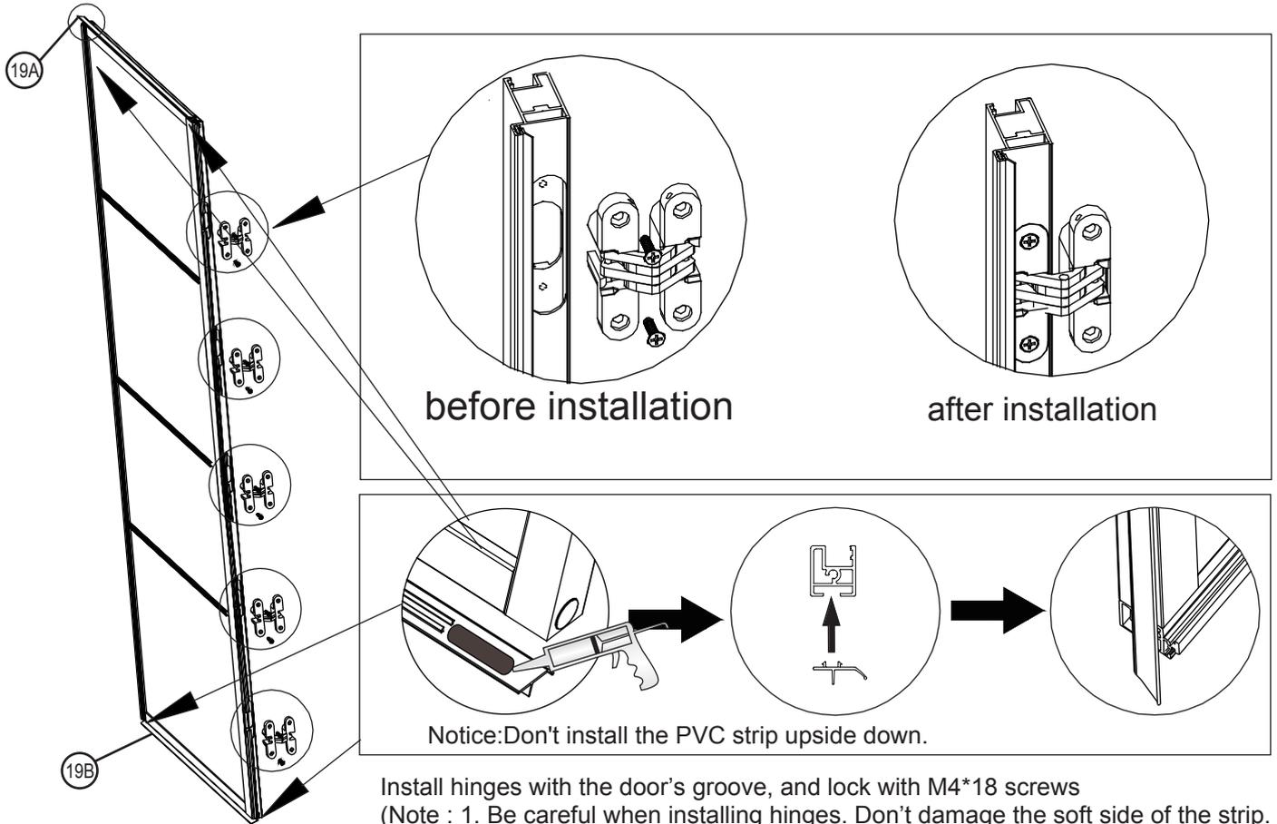
Install hinges with the door's groove, and lock with M4\*18 screws
