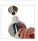
Temporarily cap off the end of the shower arm and turn on the shower to pressurise the system and check for leaks. If all is sound, turn the shower off and remove the blanking cap (remembering the system may be under pressure).
