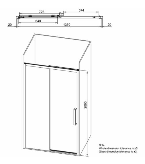
ISLSC1400A - Infinity 1400 slider single door stainless steel Box A
