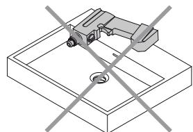
During installation one has to prevent damaging the surface of the product due to placing hard objects on the product.
