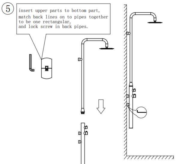
insert upper part to upper holder, lower parts to the two brass connectors, then tighten the screws. Connect the seperate shower head if have, and instal handshower and hose to hose inlet, then all installations are done.
