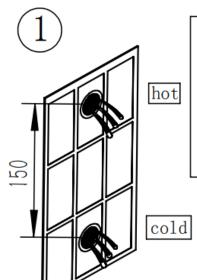
Make sure cold & hot water pipes installed at 1050mm height. Flush the pipes before installation.
