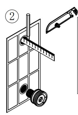
Measure the depth of the inner thread of cold & hot water pipes and mark it.
