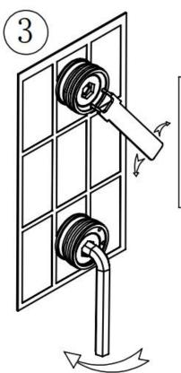
Fit the two brass connectors to the stainless fixing plate with two holes.
