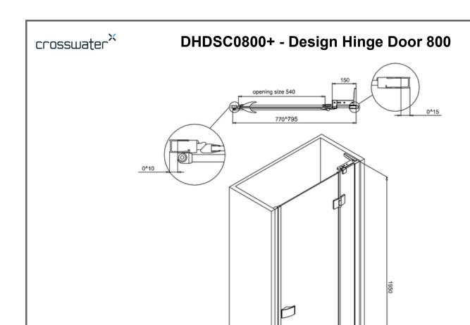
Whole dimension tolerance is ±5. Glass dimension tolerance is ±2.
