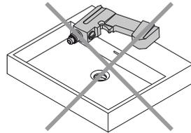
During installation one has to prevent damaging the surface of the product due to placing hard objects on the product.
