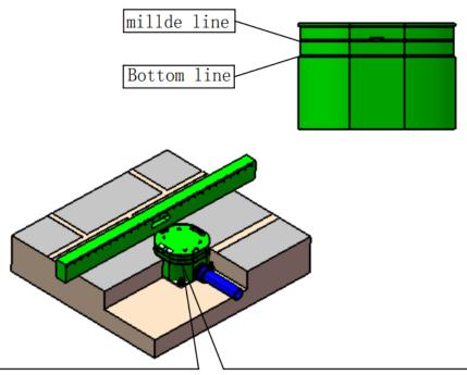
Make sure C-box is vertical and centered to you. Tighten up C-box to hole bottom with 4pcs M8 expansion screws, make sure floor tile must be higher than bottom line and lower than middle line of C-box.
