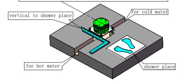
(2) Connect hot and cold water pipes to the embedded C-box, make sure no leaking.
