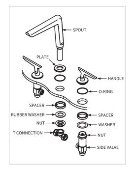
Fix the side valves to the basin, securing with the handle assemblies from the top and the spacers (if necessary), washers and backnuts from the bottom. Confirm that water exits on side valves are pointing to the center. Handles should be pointing outwards when closed and torwards you when open.
