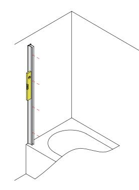
Place wall channel in position on the bath (20mm in from the edge of the bath), use a spirit level to ensure that it is vertical, and mark all 4 fixing holes on the wall.
