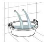
Carefully clean the water pipes before installation
