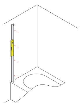
Place wall channel in position on the bath (20mm in from the edge of the bath), use a spirit level to ensure that it is vertical, and mark all 4 fixing holes on the wall.
