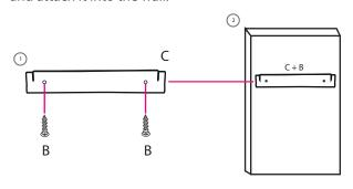
Step 2. Put the plugs into the wall.
